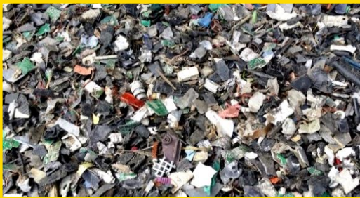
Electronic Waste with Liberated Metals
