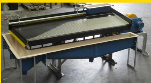
Gravity Concentration with Table
